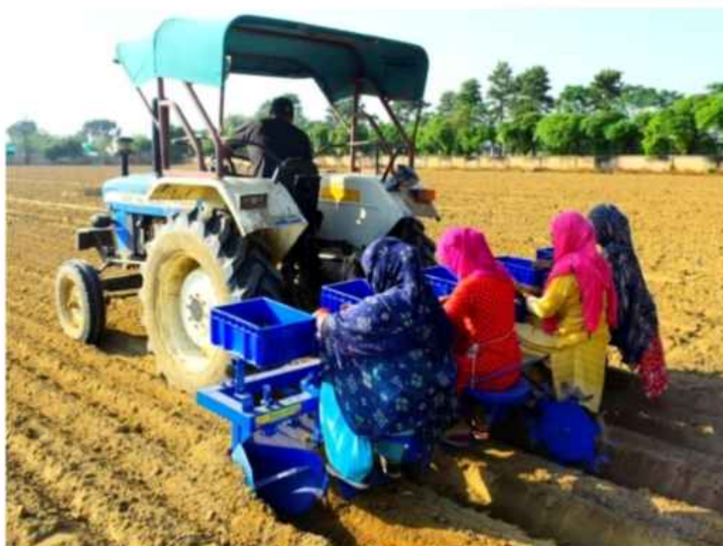
Fig. 1: Tractor operated semi-automatic potato minituber planting system
