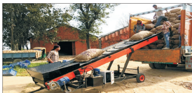
Fig. 24: Conveyor for potato loading and unloading
